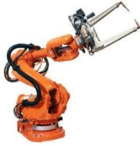
**Fig. A.8. MIG/MAG welding robot**
